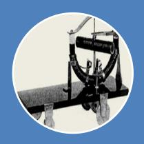
In 1828 Ányos Jedlik created a small model car powered by his new motor
